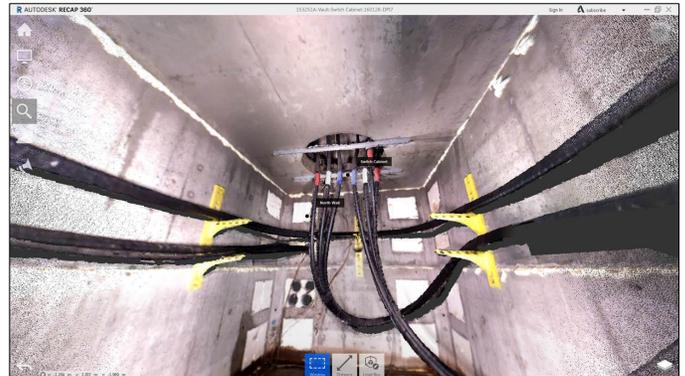
The resulting point cloud models have improved the efficiency and accuracy of the design process for ML&P. These models are used to take internal measurements, verify conduit and conductor configurations, verify equipment statuses and locations, and as an accurate 3D reference in AutoCAD, allowing engineers to design to accurate real world conditions.
